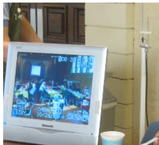
ATV in use at SVECS breakfast meeting, note J-pole on right for receiving antenna
